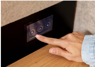
Touch screen with intensity control for general light, vanity light levels, and ventilation airflow rate
