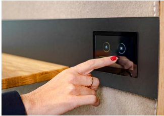
Touchscreen to regulate light and ventilation
